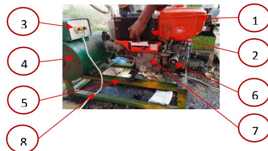
Gambar 3.1 Mesin diesel- Generator Set
