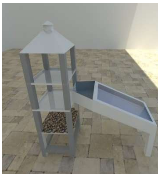
Gambar 2.1 Alat Pengering Surya Kolektor Type Hybrid
